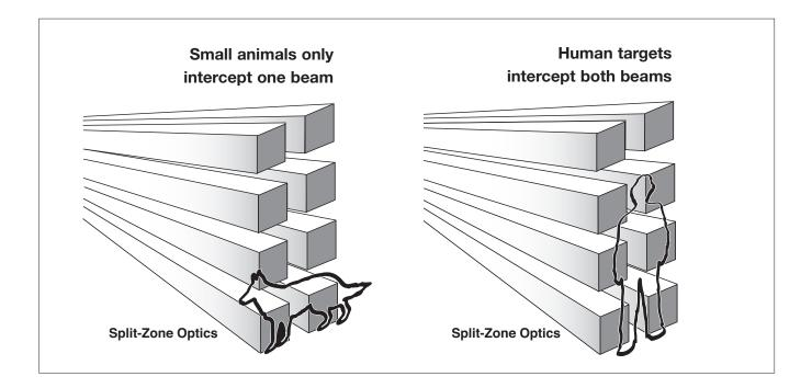
**Split-Zone Optics** splits each into two stacked sub-zones. Each sub-zone is the same size as the original, but only has about half the sensitivity. To generate an alarm, target must intercept both sub-zones simultaneously. A human target is sufficiently large enough while pets up to 40 lbs., remain undetected.
