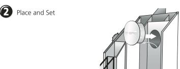
Insert the 5800MICRA's antenna into the extrusion hollow then press the transmitter body into the cored opening. Insure that the antenna moves freely in the window channel during installation.
